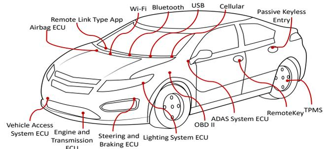
Figure 1: Automotive attack surfaces.
