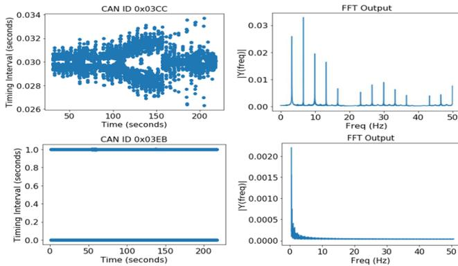
**Figure 6:** On the left side there are two examples of CAN messages with irregular timing intervals. The right side shows their respective FFT outputs. Variations in the message timings can affect the FFT output.
