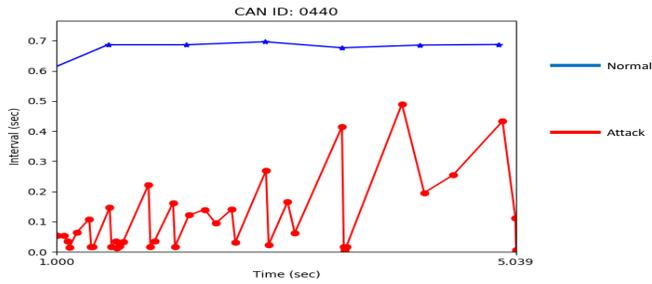
**Figure 3: Demonstrating message injection attacks affecting the timings of messages. The simulated attack messages have fluctuating message timings and are shorter than normal depending on rate of injection.**
