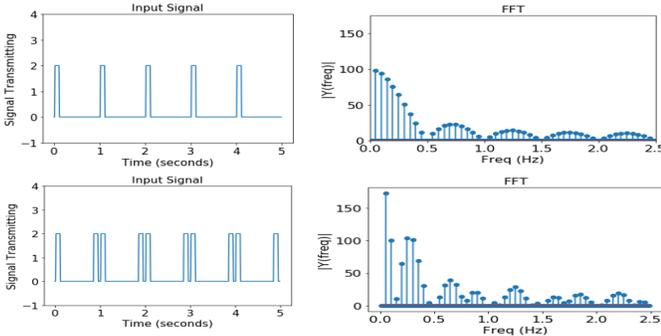
**Figure 7:** As the message rate doubles during injection attack, the magnitudes of certain frequency peaks will increase.
