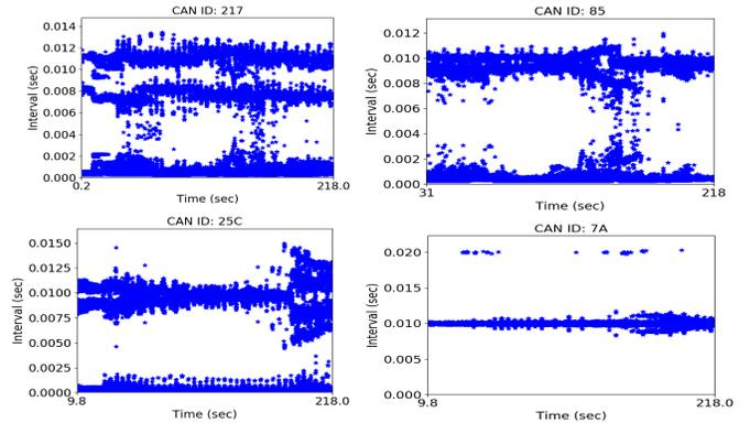
**Figure 4: Multiple CAN messages show varying message intervals. Some messages show multiple distinct intervals while some vary due to changes in vehicle operations.**
