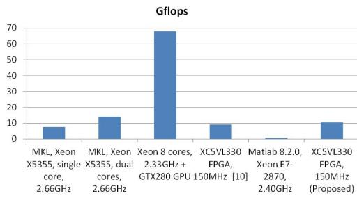
Fig. 6: Performance comparison with single core, multi-core, GPU and recent FPGA work.
