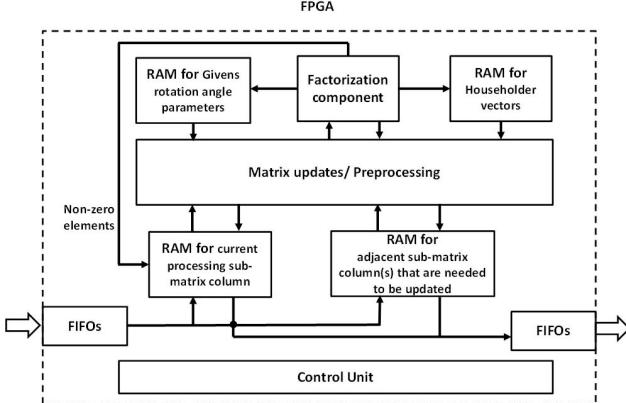
Fig. 2: Block diagram of our Hybrid QR decomposition architecture.
