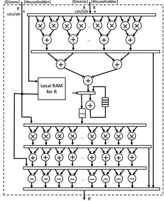
Fig. 3: Matrix updates/preprocessing component architecture.
