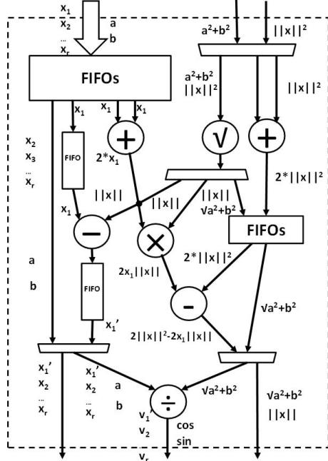
Fig. 4: Dataflow view of the factorization component.
