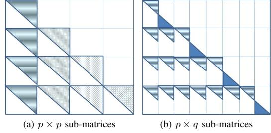
Fig. 1: An example sub-matrix partition of an  $m \times m$  matrix for our Hybrid QR decomposition algorithm
