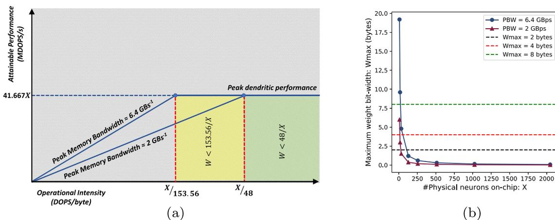
Figure 7 a Roofline analysis of CyNAPSE routing performance and b compute-bound performance requirements for CyNAPSE routing cycle.
