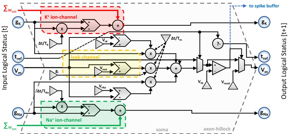
Figure 4 The full-custom digital generalized integrate and fire neuron.
