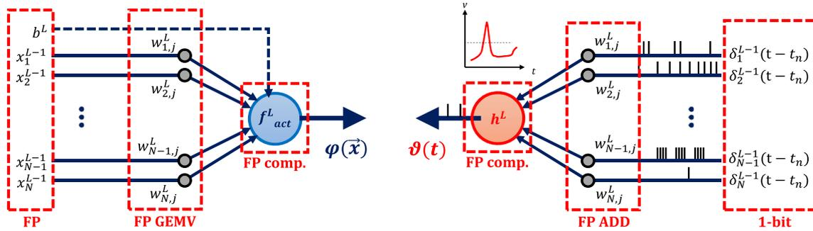
**Figure 1** Schematic descriptions of a typical perceptron or artificial neuron (left) compared to the working of a spiking neuron (right) in their respective networks.
