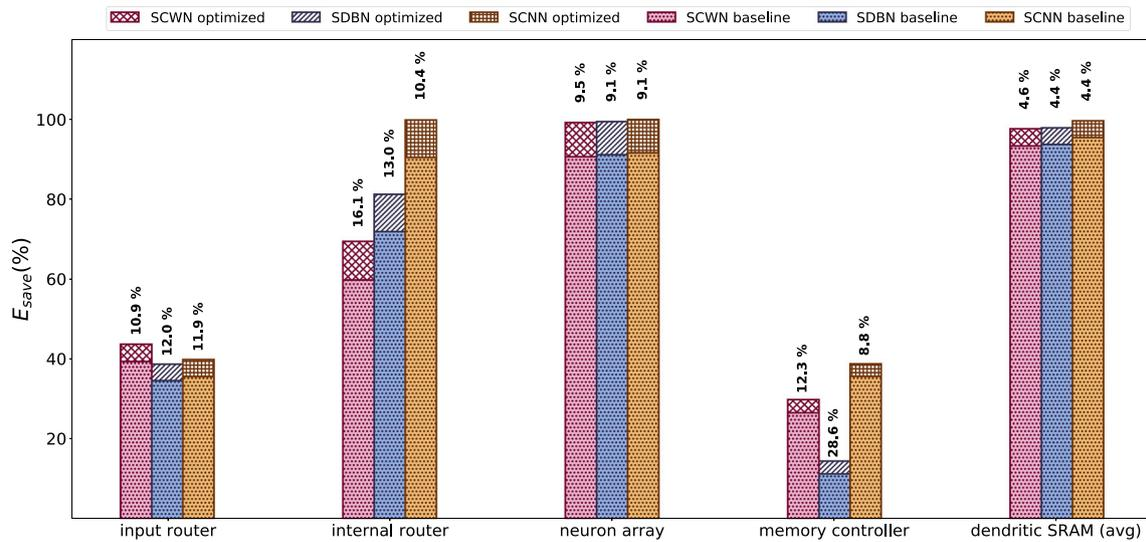
**Figure 18** Improvement in net leakage savings in every module using its optimal  $T_{idleDetect}$  for each benchmark.
