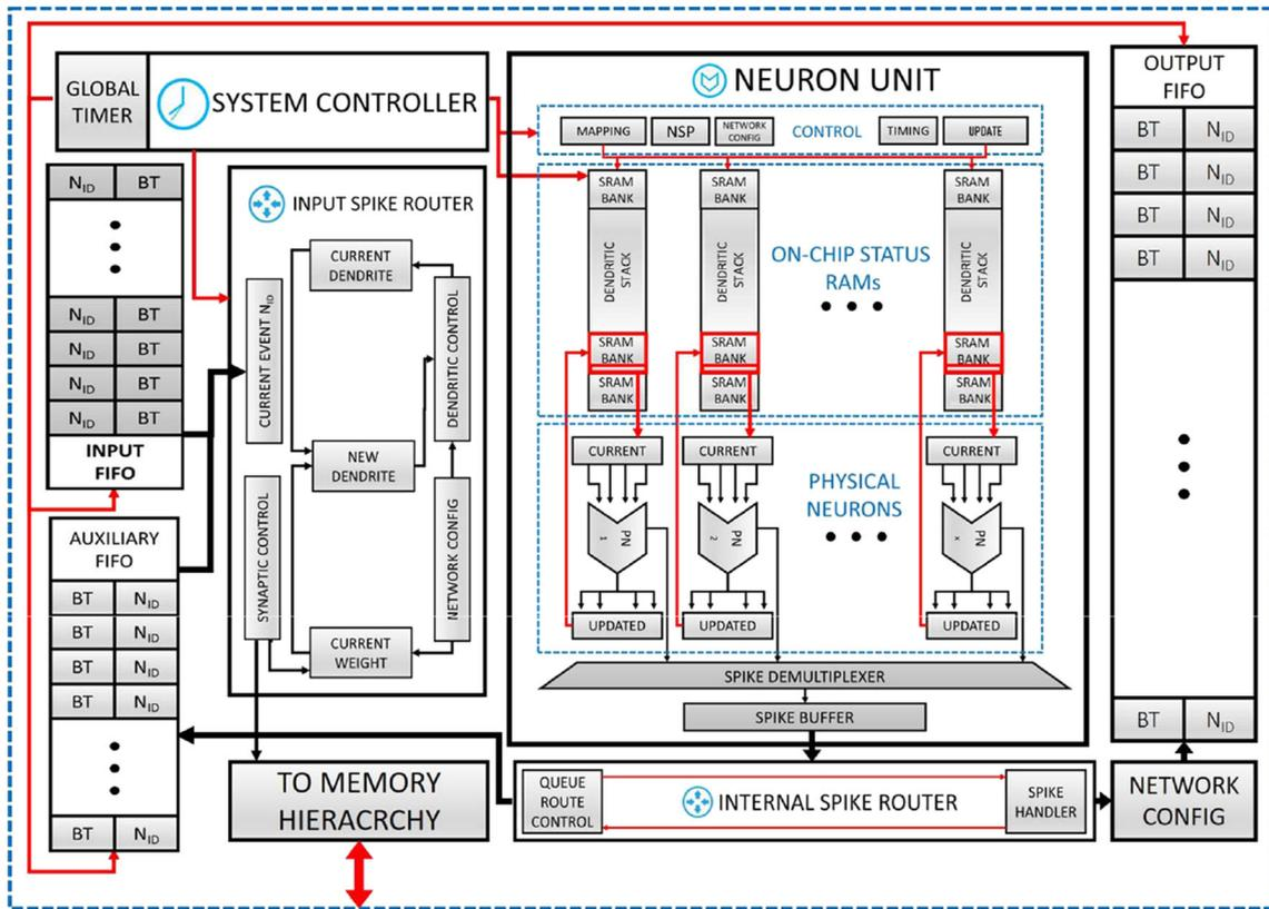
Figure 3 The overall chip microarchitecture of the CyNAPSE neural accelerator.
