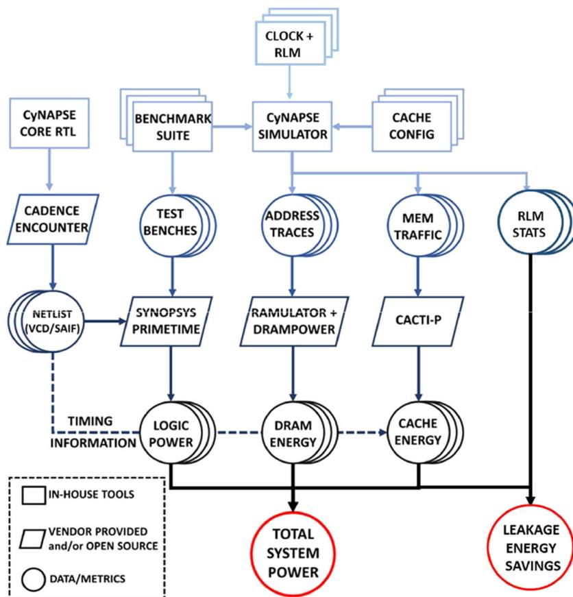
All our on-chip SRAM structures were bypassed from the CAD process and modeled only for functional verification. For estimating timing and power of SRAMs we used CACTI-P [43].
