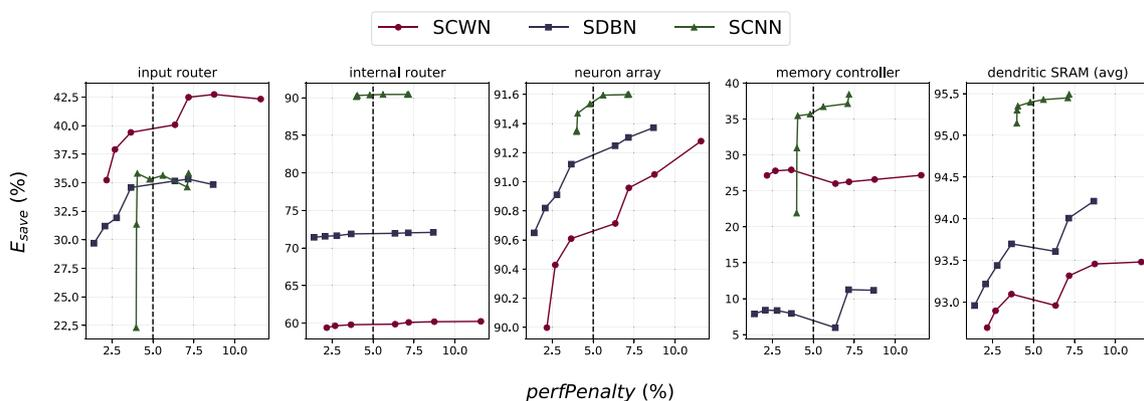
**Figure 17** Net savings in leakage energy against net performance penalty incurred as  $T_{idleDetect}$  is varied for each benchmark and hardware macro.
