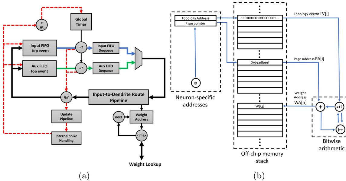
**Figure 5** **a** Control flow of SNN emulation in the CyNAPSE Core and **b** Control flow of a single synaptic weight lookup by the input router.
