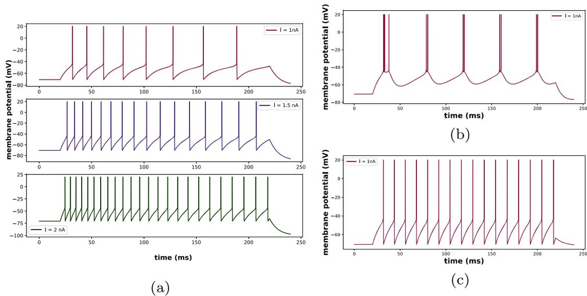
**Figure 2** Simulation characteristics of the LIF neuron showing membrane potential traces in **a** regular spiking, **b** tonic bursting and **c** fast spiking behaviors.
