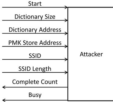
Fig. 3. Attacker input and output interface.
