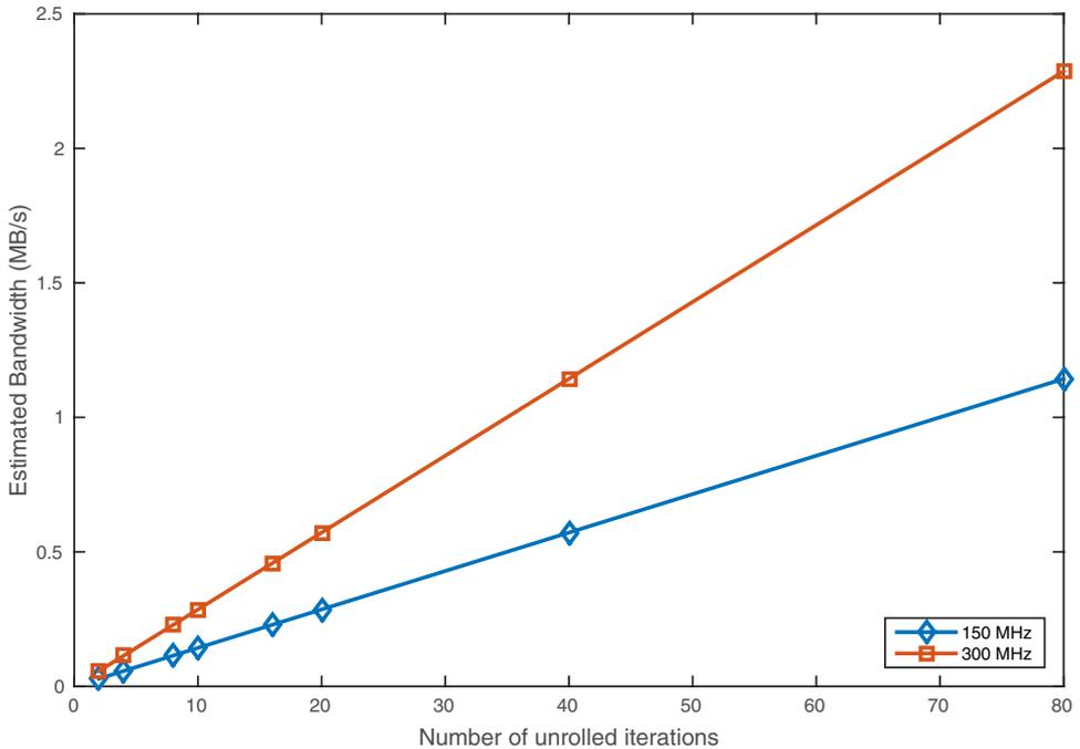
Fig. 12. Estimated bandwidth of the complete design, in MB/s.
