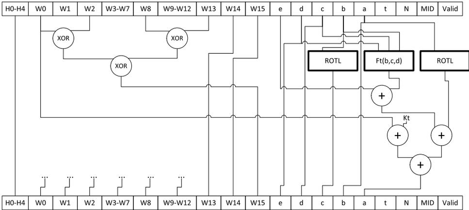
Fig. 9. The SHA-1 inner loop pipeline stage.
