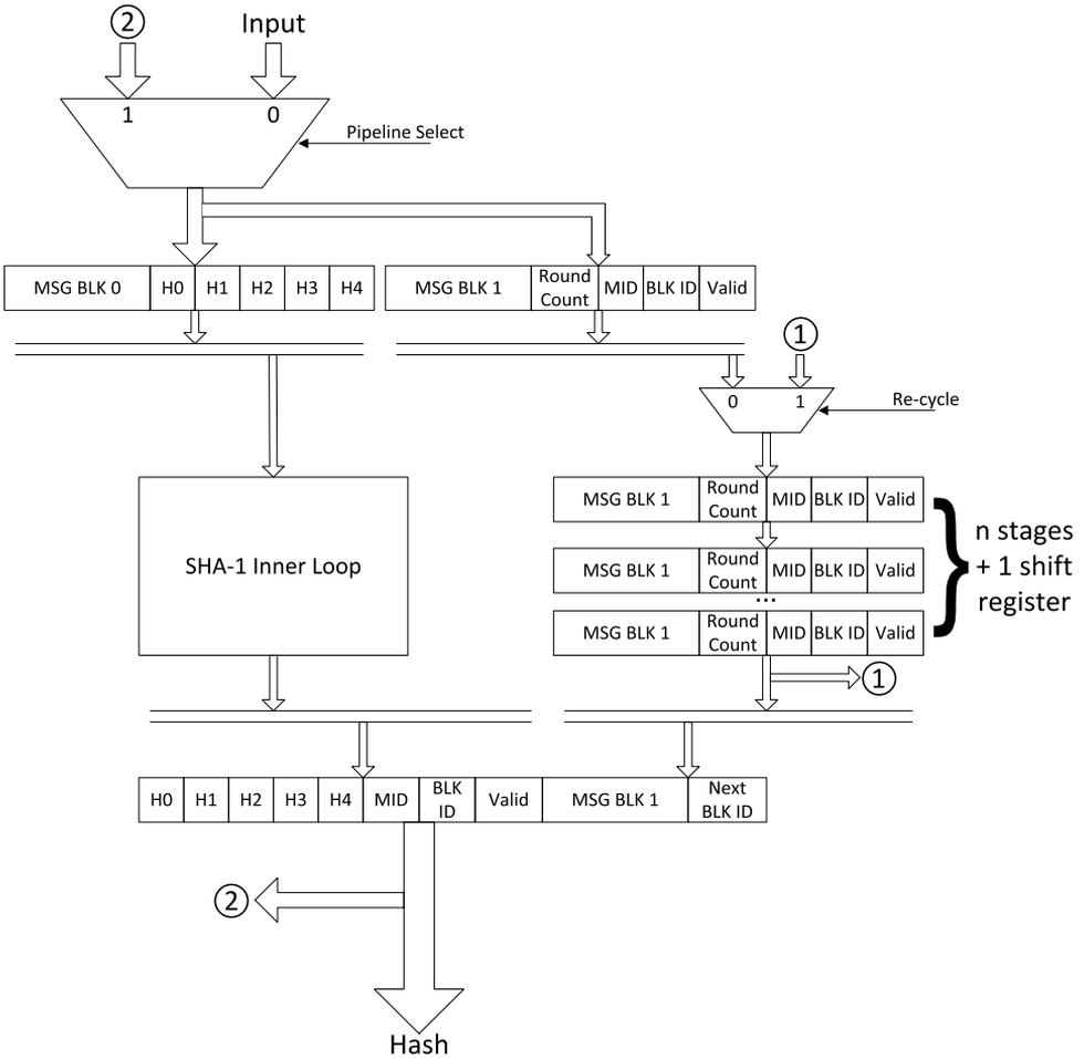
Fig. 8. Top-level view of the SHA-1 component.
