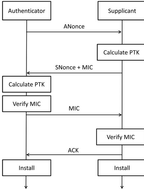
Fig. 1. The four-way handshake.
