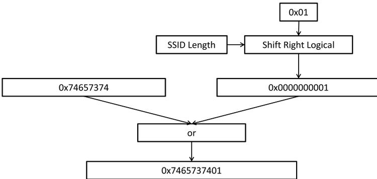
Fig. 6. Round 1 T generation using “test” as the SSID.
