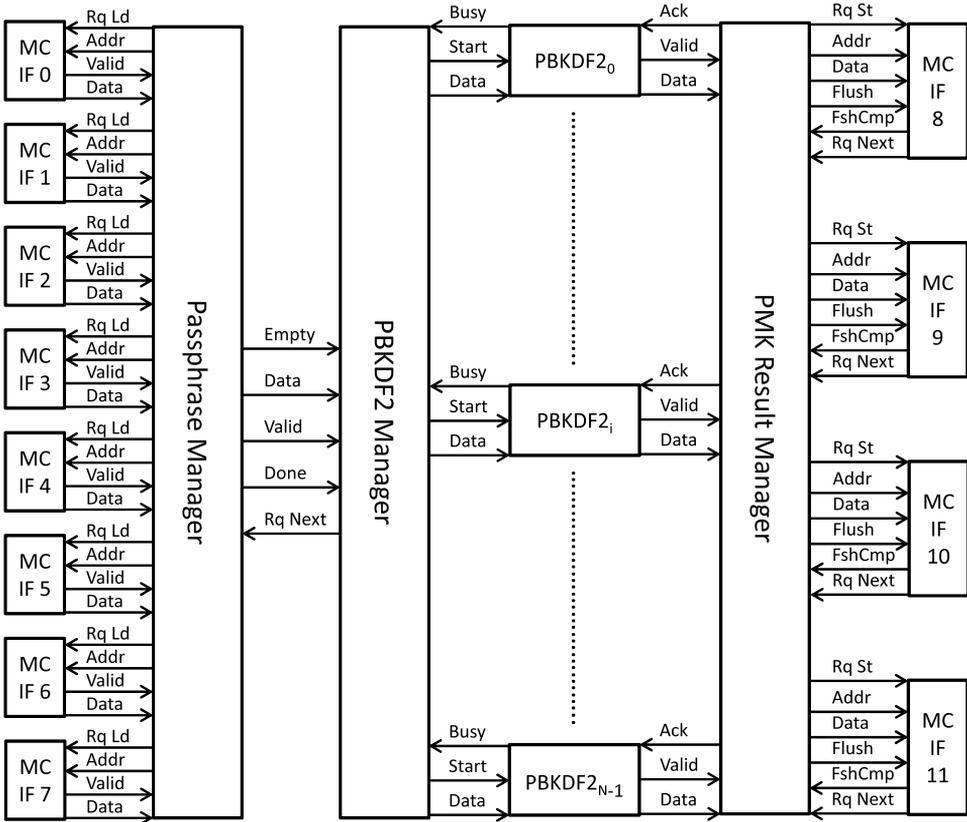
Fig. 4. High-level view of our attacker architecture.
