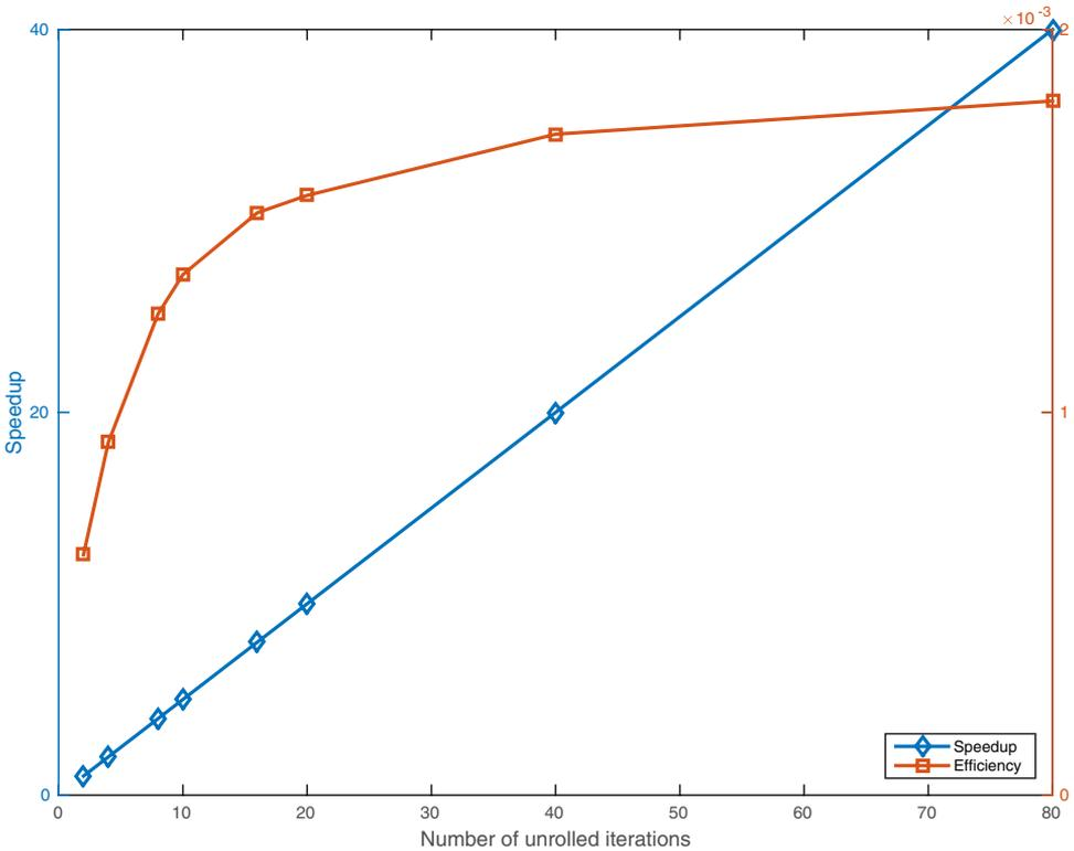
Fig. 10. Speedup and efficiency of the SHA-1 implementation.
