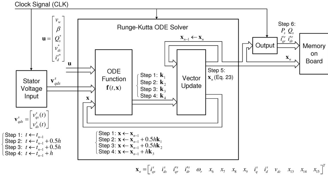
Fig. 2. FPGA implementation of DFIG wind turbine system
