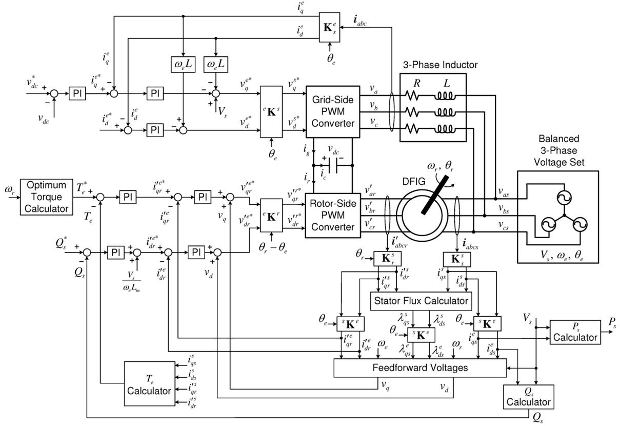
Fig. 1. Control block diagram for DFIG
