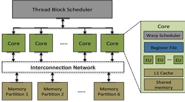
Fig. 2. Block diagram of GPU hardware
