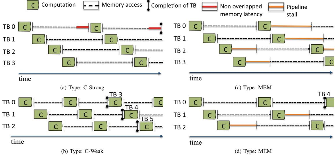
Fig. 4. Depiction of memory latency tolerance for different kernel categories.
