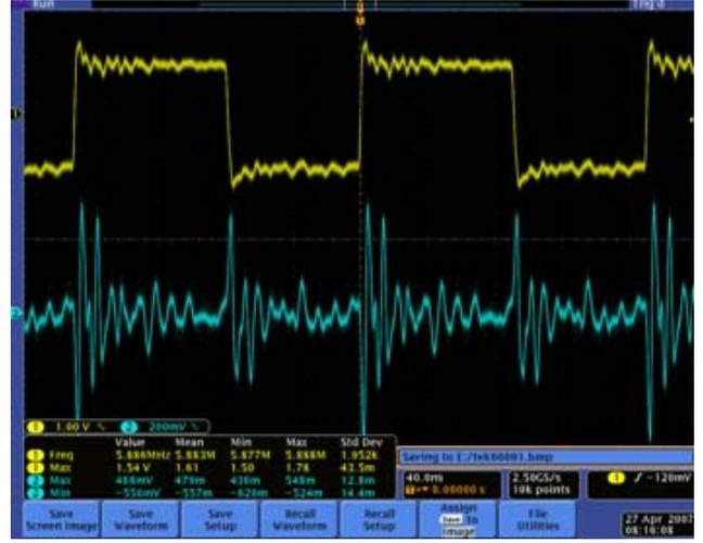
Fig. 6. Power traces for four DES iterations in one trigger pulse period
